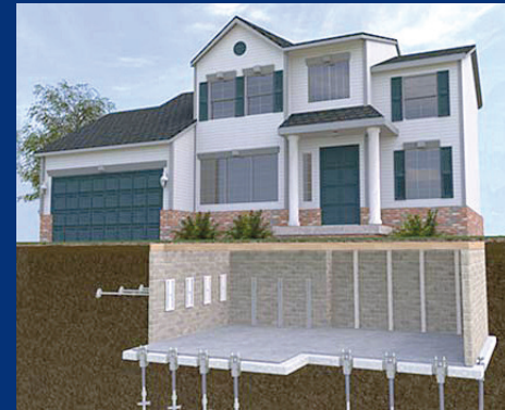
STRUCTURAL FOUNDATION LIFTING
